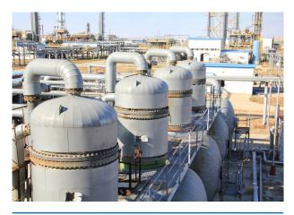
Figure 3. A typical multi-stage FIBER FILM Contactor and separator system treating light crude oil in a stick built unit.
