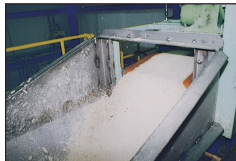
The LO-CAT II system converts H 2 S to a harmless sulfur cake.
